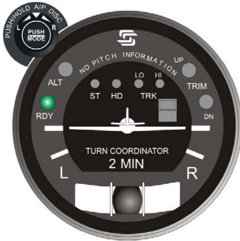
Fig. 2-3. AP Display, RDY for Operation (System Twenty)
