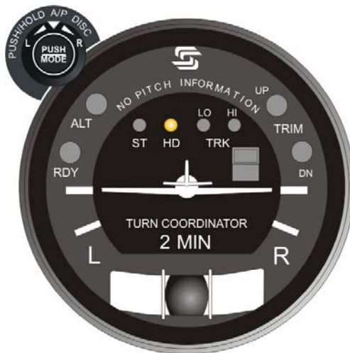
Fig. 2-18. AP Display, HD Mode Engaged (System Twenty)
