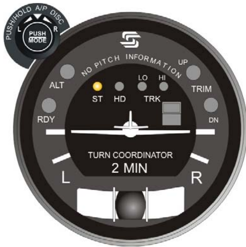
Fig. 2-21. AP Display, ST Mode Engaged (System Thirty)
