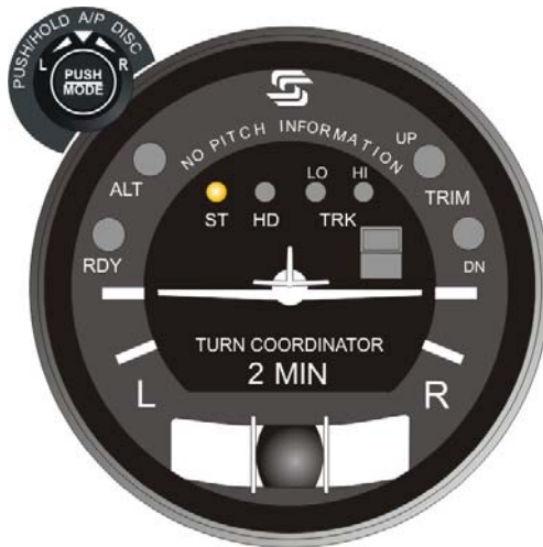
Fig. 2-17. AP Display, ST Mode Engaged (System Twenty)
