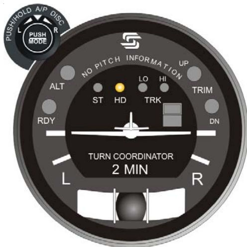
Fig. 2-22. AP Display, HD Mode Engaged (System Thirty)
