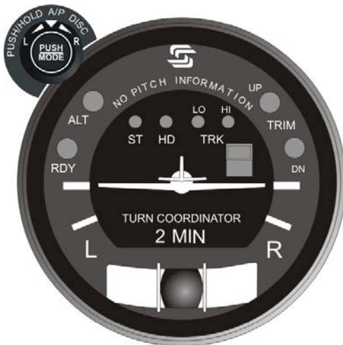
Fig. 2-2. AP Display, All Lamps Extinguished (System Twenty)
