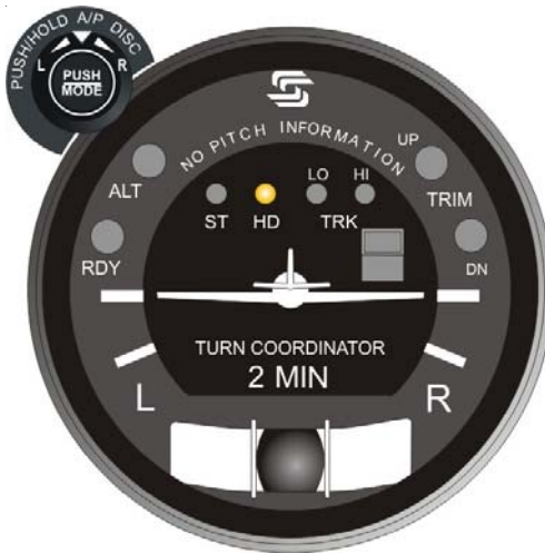
Fig. 3-2. AP Display, HD Mode Engaged
